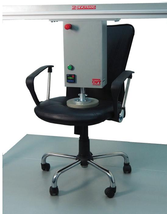
USED TO TEST DURABILITY OF CHAIRS, ARMCHAIRS
